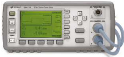
Figure 14. E4417A power meter configured to show a trace display (upper window) and a dual numeric display (lower window).
