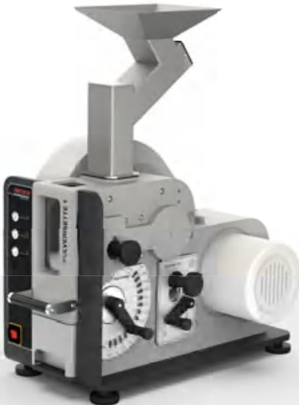
Comminution of ferrous alloys with the Jaw Crusher PULVERISETTE 1 premium line – 6.5 mm gap width
