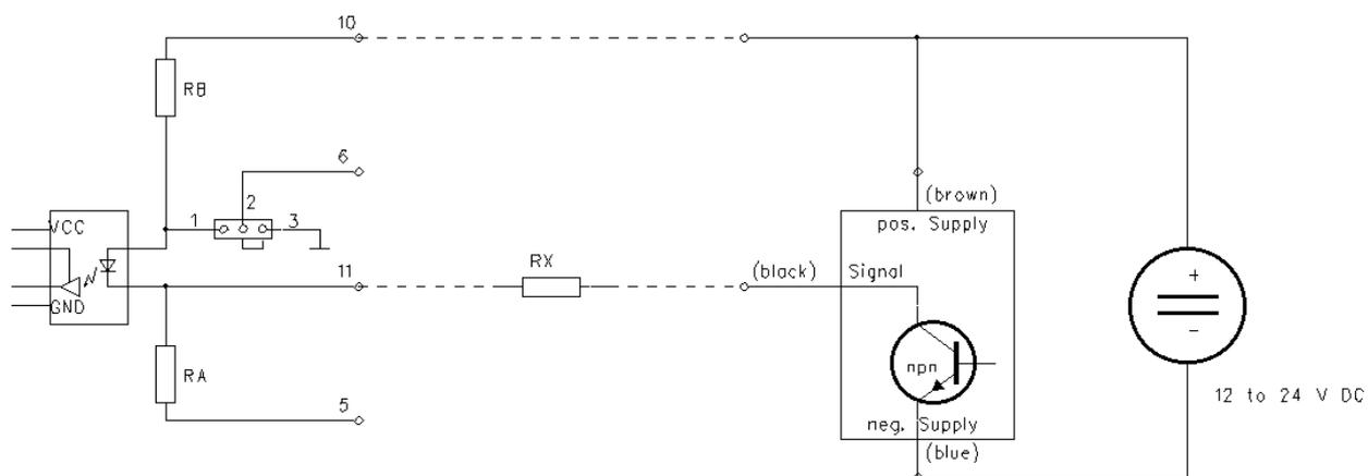
Resistor RX must be built into the connection between the light barrier and the parallel plug.
