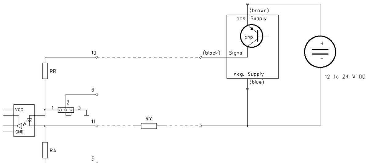
Resistor RX must be built into the connection between the light barrier and the parallel plug.
