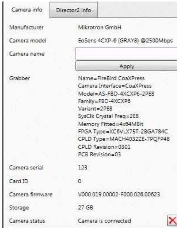
Camera Info panel showing link speed 2500 in line “Camera model”.
