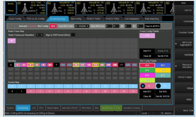
Figure 5. Scheduling Map tab to configure the resource allocation for the selected cell
